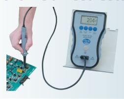
Trek's Model 821HH Infinitron® Hand-Held Electrostatic Voltmeter represents the next generation of contacting precision surface voltage measuring instruments, providing input characteristics far beyond the limits of any currently available hand-held voltmeter product.
