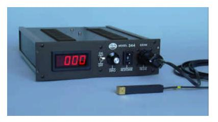
Measurement Range: 0 to ±2 kV DC or peak AC
