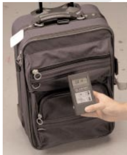
palmRAD 907 shown above. Used to locate radiation and measure in \mu R.
