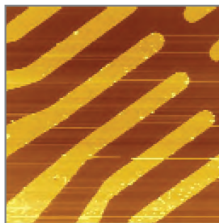
10 X 10 micron image of silicon sample with gold pattern. At the left is a topography image at the right is a conductive AFM image. Two of the "fingers" on the test pattern are grounded and show contrast in the conductive AFM image
