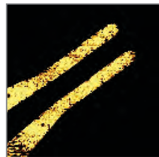
10 X 10 micron image of silicon sample with gold pattern. At the left is a topography image at the right is a conductive AFM image. Two of the "fingers" on the test pattern are grounded and show contrast in the conductive AFM image
