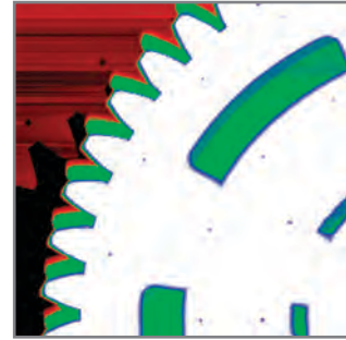
40 X 40 micron image of a gear fabricated with MEMS.
