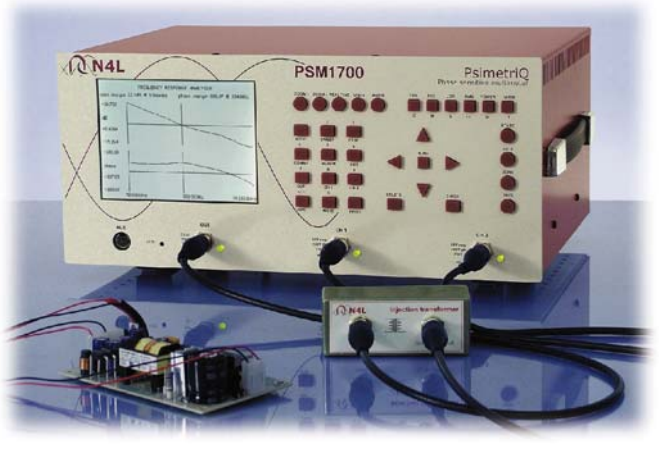
PSM1700 with N4L injection transformer testing an SMPS
