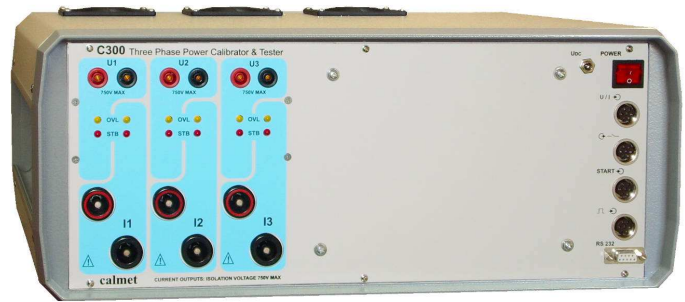
C300 3- phase source up to 120A (1- phase up to 360A) and 560V
