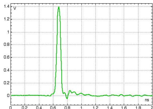
50 ps impulse response (0.2ns/div) Generator is PSPL 4015B pulser
