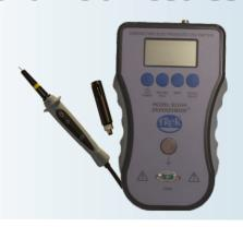
Trek's Model 821HH Infinitron® Hand-Held Electrostatic Voltmeter represents the next generation of contacting precision surface voltage measuring instruments, providing input characteristics far beyond the limits of any currently available hand-held voltmeter product.
