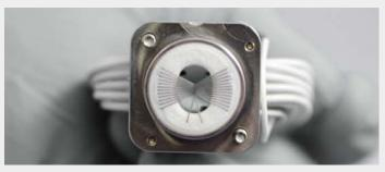
TV19 VersaTile<sup>™</sup> probe cards are designed with Celadon's patented ceramic technology for superior electrical performance, yet is highly modular due to it's 28mm x 28mm chassis.
