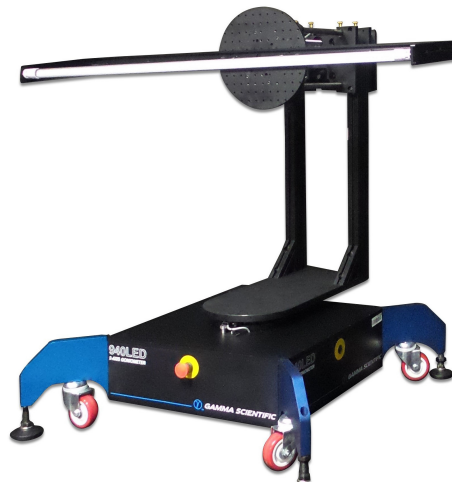
Gamma Scientific 940 LED Goniometer Measuring an LED T8 Tube Light
